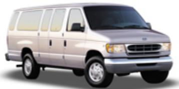
Adding passengers and cargo causes the center of gravity to move upward and rearward, increasing a vehicle's tendency to roll over and increasing the potential for the driver to lose control in emergency maneuvers. Fifteen-passenger vans are three times more likely to roll over when loaded with more than ten passengers.
